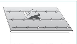
Multiple 2" x 6" roof brackets and slide guards, properly spaced can stop a worker from sliding off a steep roof. Make sure all roof brackets and slide guards bear on solid surfaces.
