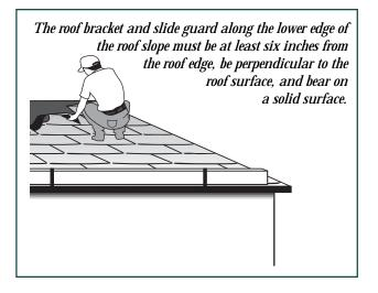
• The roof bracket and slide guard along the lower edge of the slope must be at least six inches from the roof edge and perpendicular to the roof surface. Other brackets and slide guards above the lower edge may be installed at a 60-degree angle to the roof surface. *All roof brackets and slide guards must bear on solid surfaces.*
