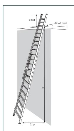
Key points for ladder safety: Angle the ladder so that it has a 4:1 slope; make sure the top extends at least three feet above the roof edge; tie off the ladder so it won't tip over.
